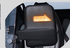
Side Mirrors with Turning Signals
